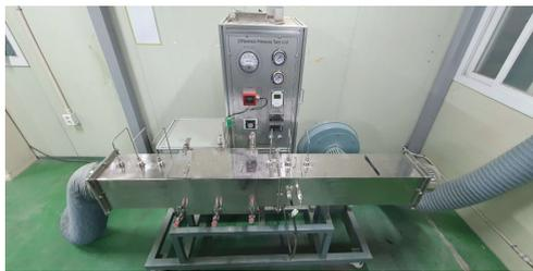
Fig. 11. Pressure drop analysis equipment.
