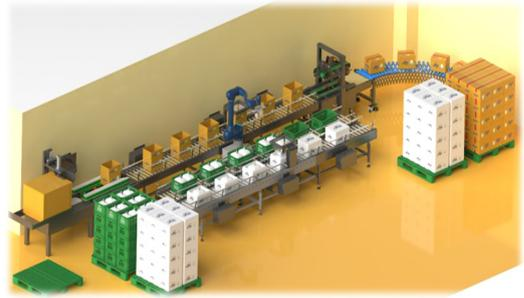
Fig. 5. Case study 2: Robot applied automated transfer stacking process
