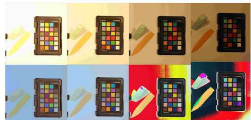
Fig. 4. Example of Color Correction using Color Patch
