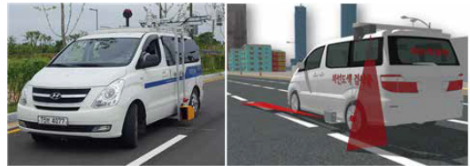
Fig. 1. Vehicle-mounted lane painting luminance and quality inspection device.
