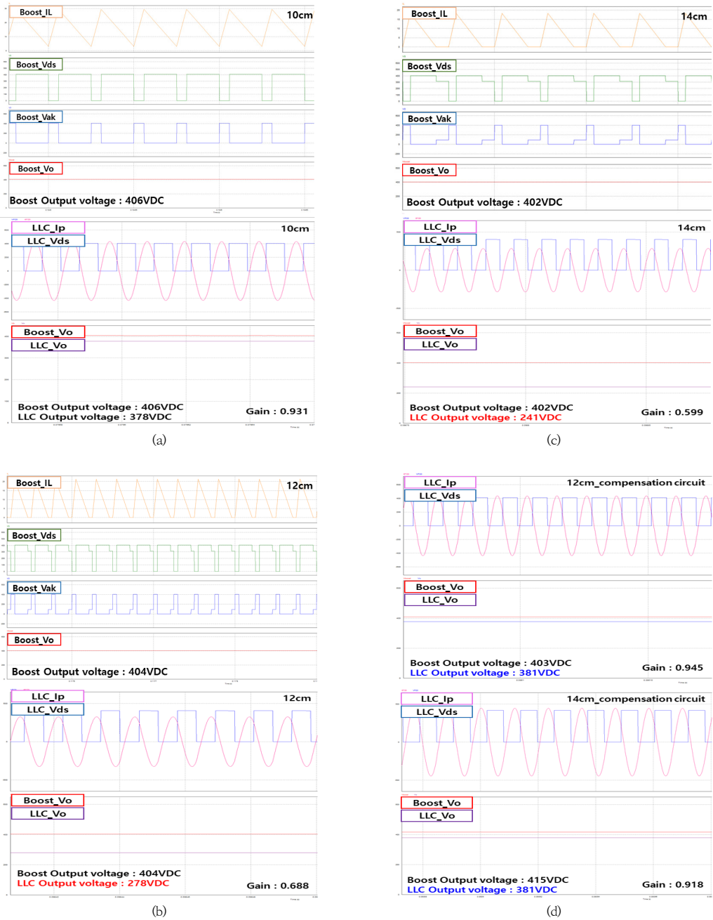
Fig. 10. Simulation of WPT resonance compensation system
