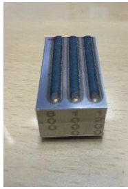
Fig. 2. Single track specimen manufactured by DED
