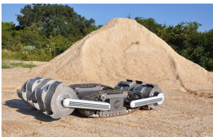
Fig. 7. Bucket drum Regolith Advanced Surface Systems Operations Robot (RASSOR)
