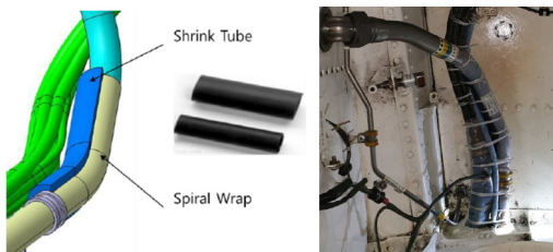
Fig. 7. Application of Shrink tube and Spiral Wrap
