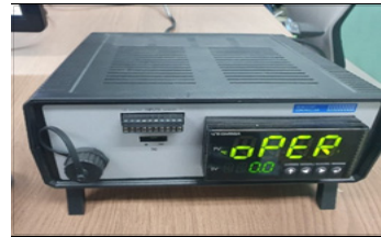
(c) temperature controller
