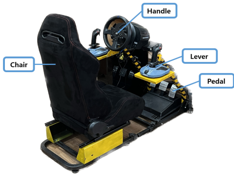
Fig. 3. Simulator hardware of wheel loader
