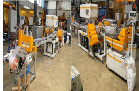
Fig. 4. Pilot sheet Extruder
