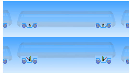
(b) Carbody bounce mode(0.81Hz)
