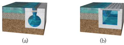
Fig. 2. Comparison of urban drainage system (a) O-shape (b) U-shape
