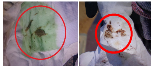
Fig. 2. Sludge in Coolant
