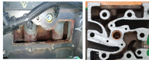
Fig. 7. Rust inside the cylinder head
