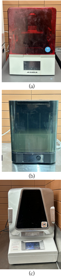
Fig. 2. 3D printing system (a) DLP type 3D printer (b) resin wash (c) resin curing unit
