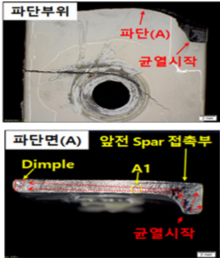
Fig. 3. Detail of Fracture A
