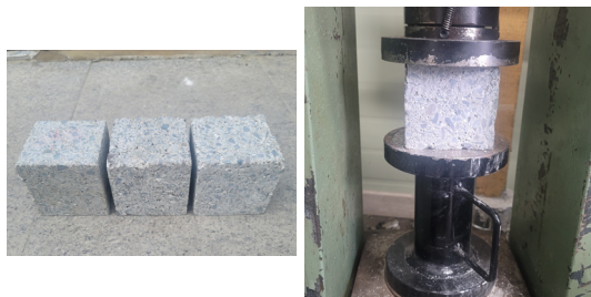
(a) Compression test specimen (b) overview of Compression test
