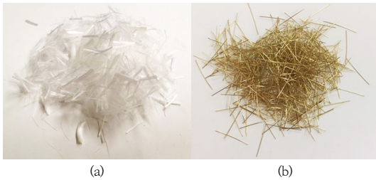
Fig. 2. Fiber reinforced materials (a) PVA fiber (b) Micro steel fiber
