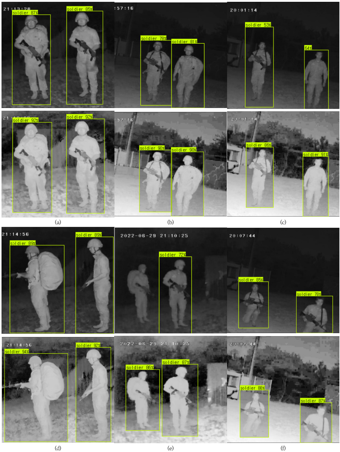
Fig. 7. Comparison of confidence score for test images (a) front posture (b) front posture (c) front posture (d) left posture (e) right posture (f) kneeling posture
