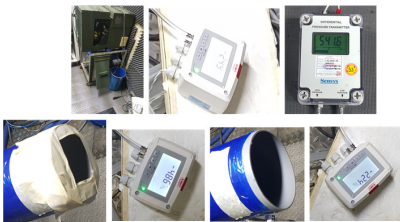
Fig. 6. Experiment of measuring cooling performance
