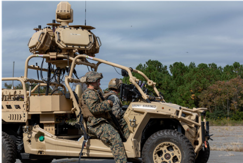
Fig. 8. Mobile-Low, Slow, Small Unmanned Aircraft Integrated Defeat System in U.S. Marine Corps
