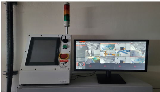
Fig. 16. Cutting Equipment Control through Remote Control
