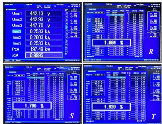
Fig. 16. Measurements results of P.F and iTHD (180kW)
