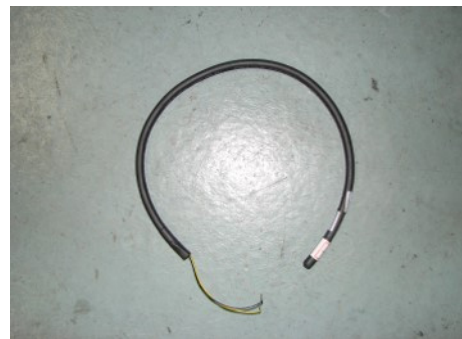
Fig. 2. Unshielded Rogowski coil samples used in the test
