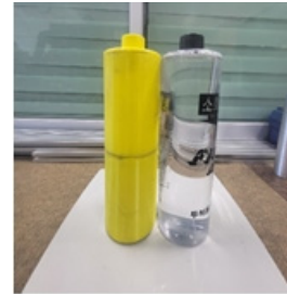
Fig. 8. Fire grenade imitation for experiment.
