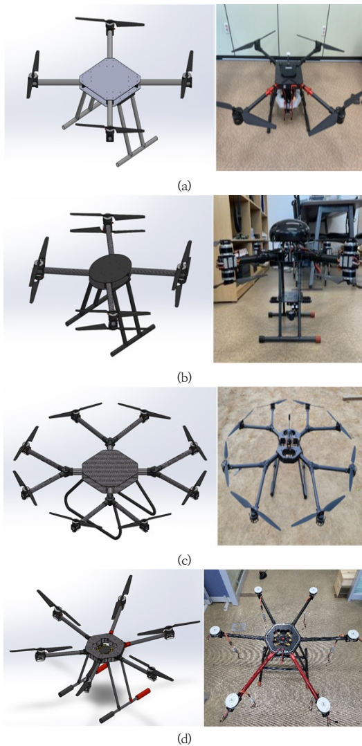
Fig. 5. Produced and reviewed drone frames. (a) Quad type, (b) X8 type, (c) Octo type, (d) Hexa type.
