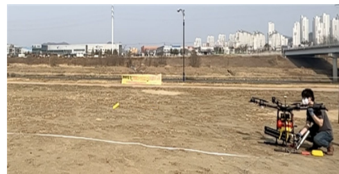
Fig. 9. The scene of the fire grenade travel distance test.
