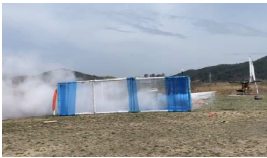
Fig. 12. Powder fire extinguisher firing range test scene.
