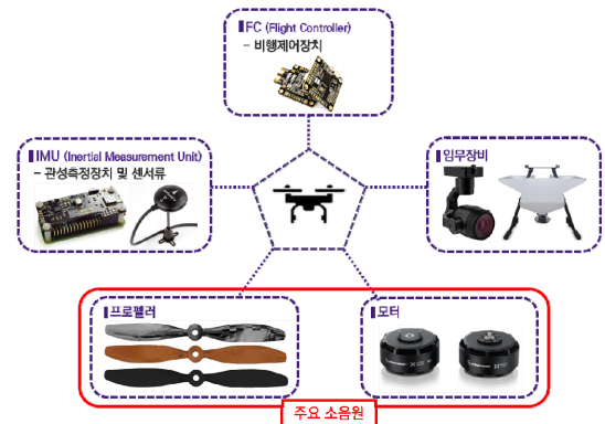
Fig. 4. Classification of Drone Main Parts and Noise Sources
