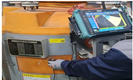
Fig. 7. Equipment of Ultrasonic testing
