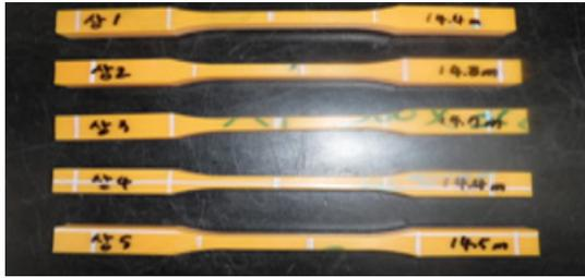
Fig. 4. Tensile test Specimen (ISO 527-4)
