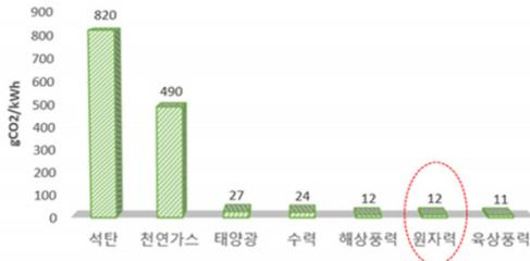
Fig. 3. Carbon emission by power source[11]
