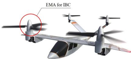
Fig. 1. EMA for IBC in eVTOL
