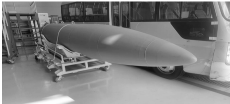
Fig. 3. Test Specimen for MMOI Measurement
