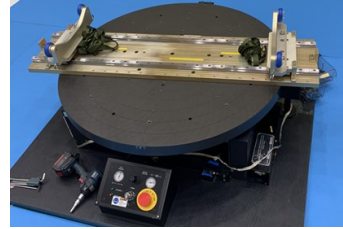
Fig. 1. Equipment for measuring MMOI of Large Structure
