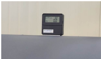
Fig. 11. Check the Level of the Test Specimen
