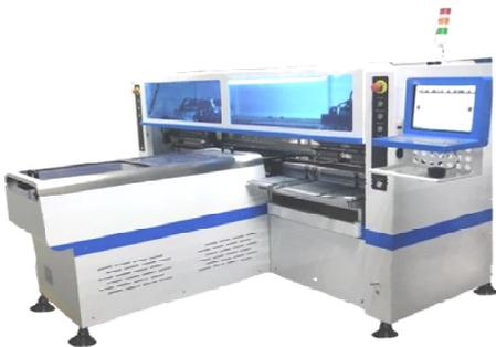
Fig. 1. Through-hole Mount Placement Machine for a PCB Manufacturing.
