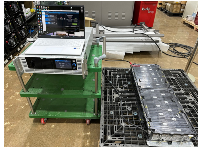
Fig. 17. Kona EV Battery and Charge-Discharge Experimental Setup
