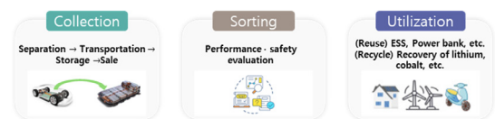
Fig. 3. Secondary Battery Reuse/Recycling Process
