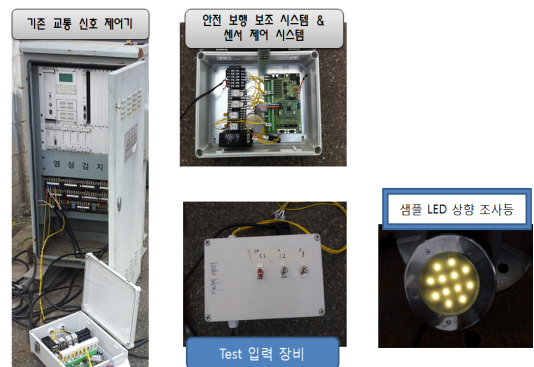
[Fig. 7] Assistive chamber system of pedestrian safety Test Equipment
