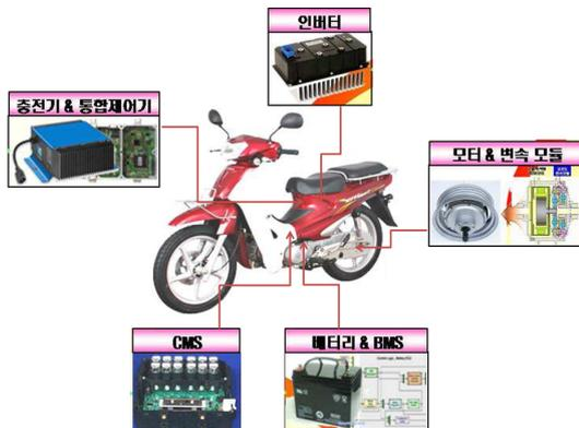
[Fig. 1] Components of electric motorcycle
