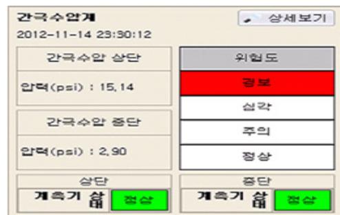
[Fig. 12] Hazard Output of Piezometer Data
