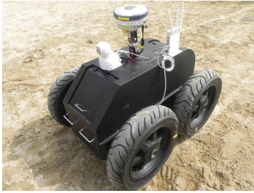
[Fig. 2] GPS Auto- Surveying system
