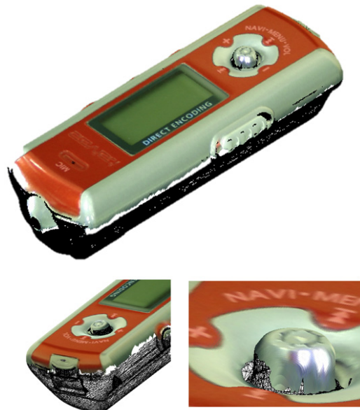
[Fig. 10] A rendering result of a texture mapped 3D model obtained by the proposed method
