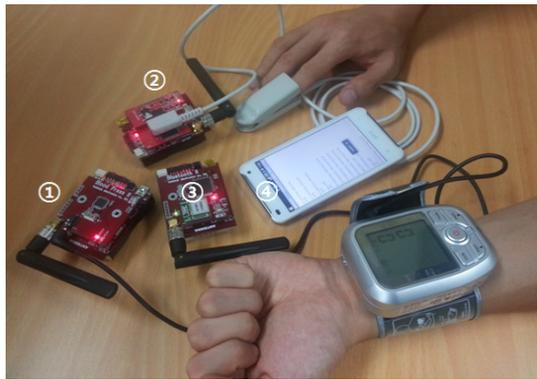
[Fig. 7] Picture of smart phone measuring DI(Dementia Index) from HRV and SpO<sub>2</sub> sensors
