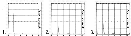
[Fig. 7] Toe crack Ultrasonic test shape(Refraction angle 70°, Back Bead)
