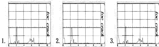
[Fig. 8] Toe crack Ultrasonic test shape(Refraction angle 70°, Back Bead)
