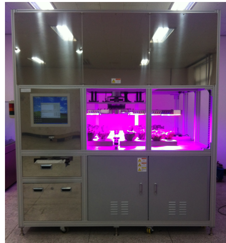
[Fig. 1] Prototype of a plant factory system containing rotational lighting system
