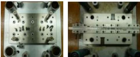
[Fig. 12] Die mould for manufacturing of the clip
