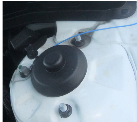
[Fig. 4] Accelerometer mounting position
