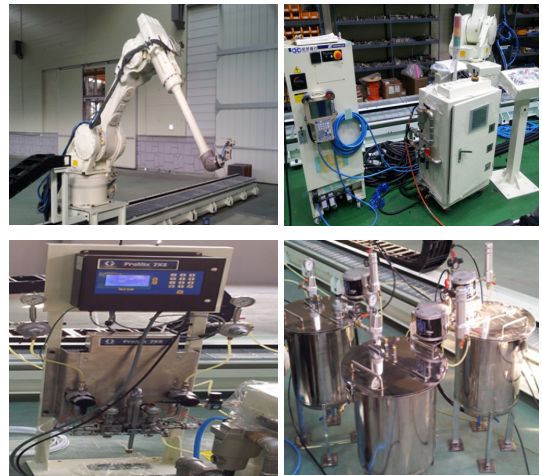
[Fig. 2] Overview of coating robot automation system developed
