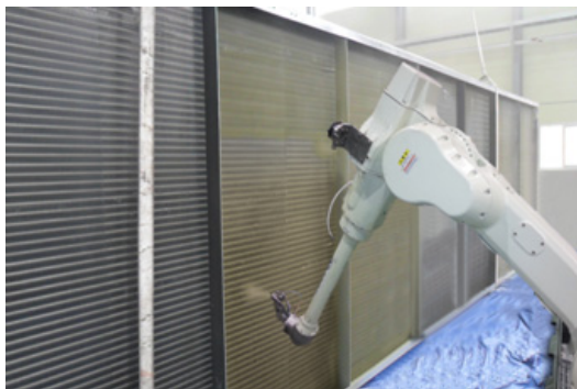
[Fig. 13] Operation view of coating robot
