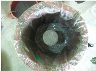
[Fig. 4] Preparation of clay layer
