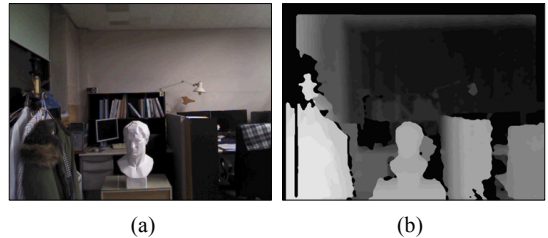
[Fig. 12] Disparity map of active camera (a) Input image (b) Disparity map
