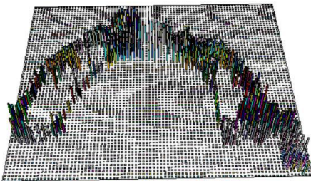
[Fig. 2] The form of sludge deposition on Hot leg Kidney Zone
