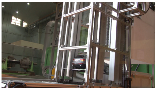
[Fig. 11] Experimental Demonstration of Vertical Transfer of a Vehicle Using the 1/10-scale Prototype
