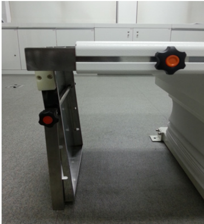
[Fig. 6] The appearance of folding the image plate holder with the X-ray table as low as possible
