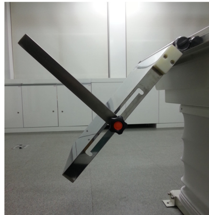
[Fig. 4] The appearance of manufactured Merchant Hun's axial viewer with X-ray table
