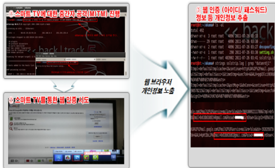
[Fig. 11] Smart TV Web Browser Authentication and Privacy Exposed Screen
