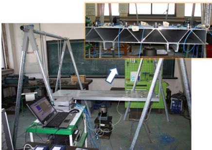
[Fig. 2] Test setup for mechanical mobility measurement of the double skin Al panel
