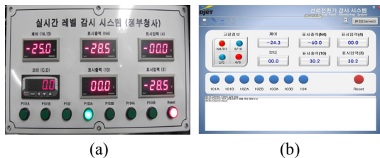
[Fig. 4] Failure detection (a) Ground failure (b) Disconnection failure
